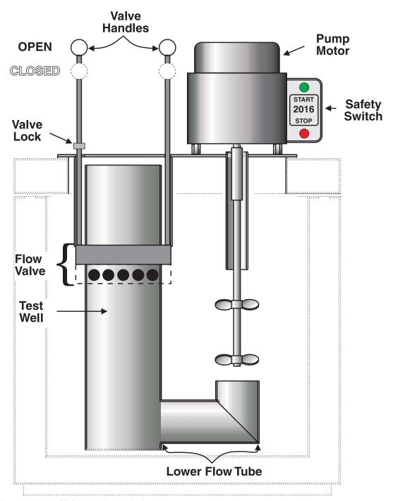
Figure 1 Typical 2016 installation in a bath
