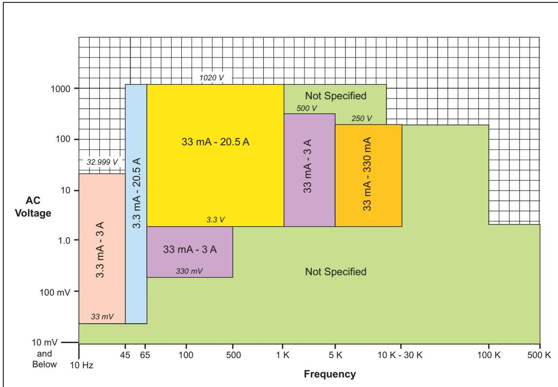
**Figure 6. Permissible Combinations of AC Voltage and AC Current for Power and Dual Output**
