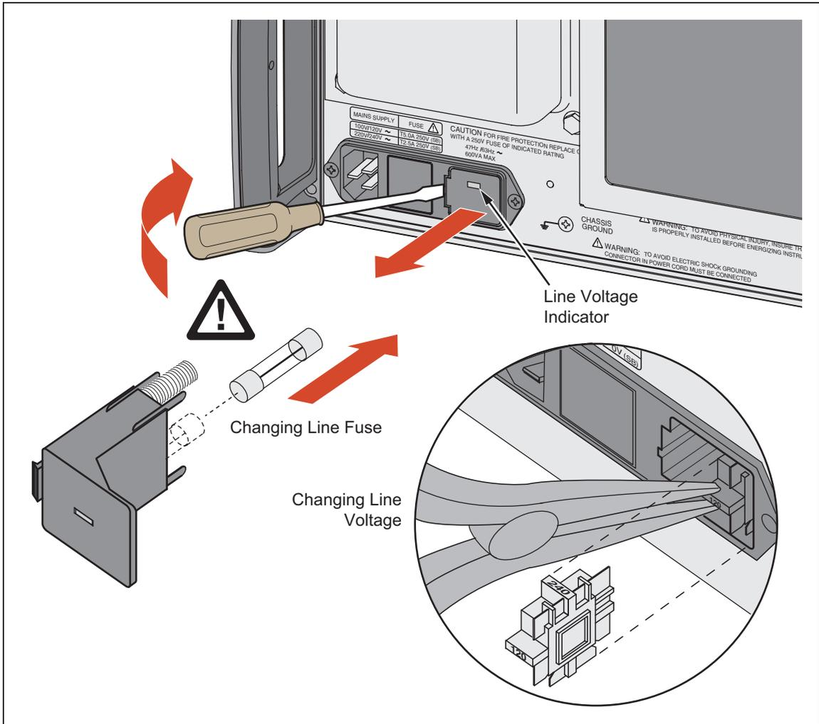
Figure 3. Access the Fuse and Select Line Voltage
