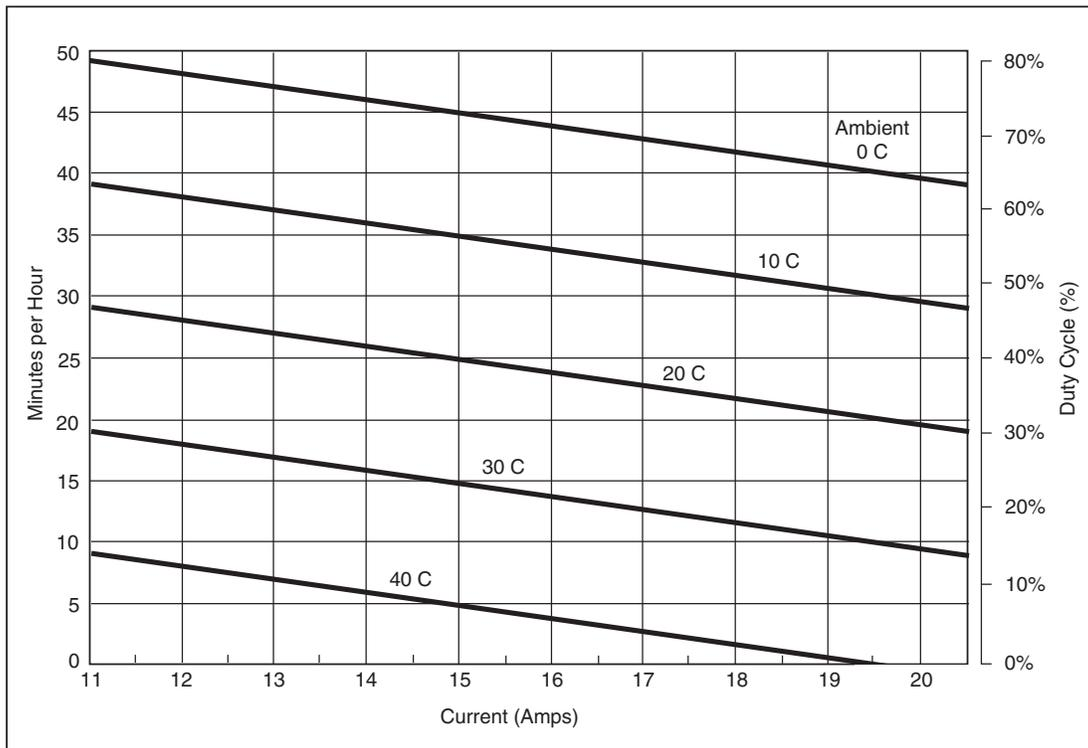
**Figure 5. Allowable Duration of Current >11 A**
