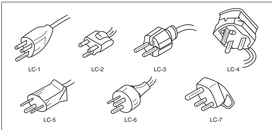
**Figure 4. Line Power Cord Types Available from Fluke**
