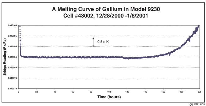
Figure 4. Typical Melting Curve of Gallium
