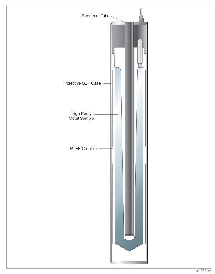
Figure 1. Construction of the Gallium Melting Point Cell
