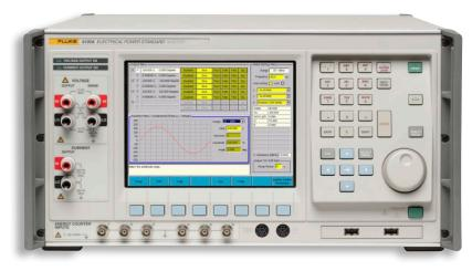
The 6105A provides the accuracy required to verify the performance of secondary standards such as those produced by Radian Research, Zera, and MTE.
