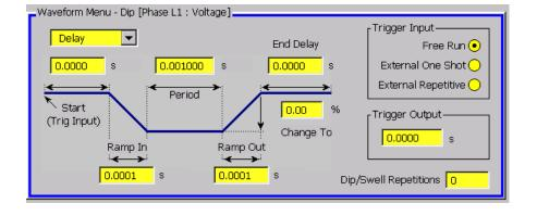
The 6105A and 6100B can be used to verify the performance of equipment used for testing immunity to voltage dips, short interruptions and voltage variations as specified in IEC 61000-4-11.
