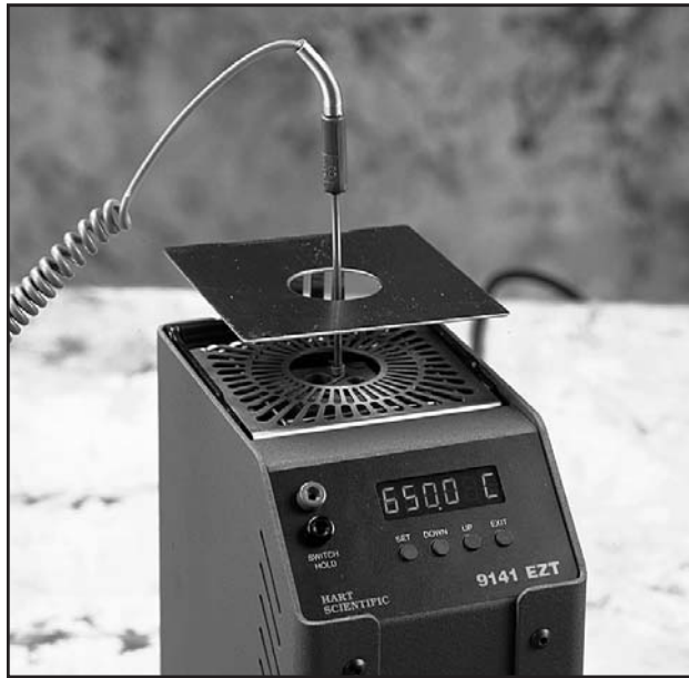
Figure 1 Heat shield installed on 9141 calibrator
