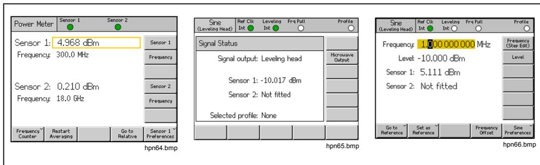
**Figure 3-34. Instrument Screens with Power Meter Readouts**
