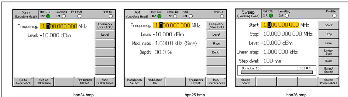
Figure 3-7. Control Screens for the RF Output Signal
