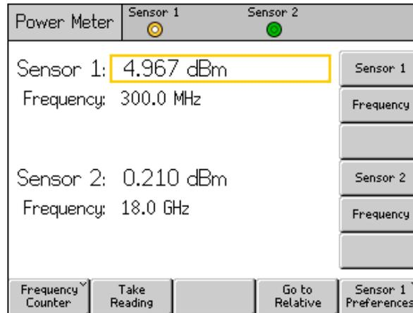
Figure 3-40. Power Meter Screen (Trigger Single Selected)
