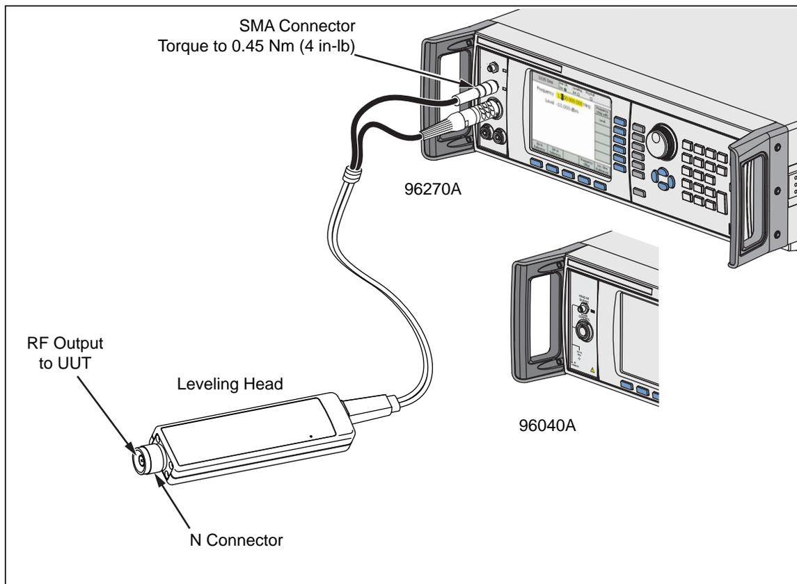
Figure 3-29. Leveling Head Output (96040A and 96270A)
