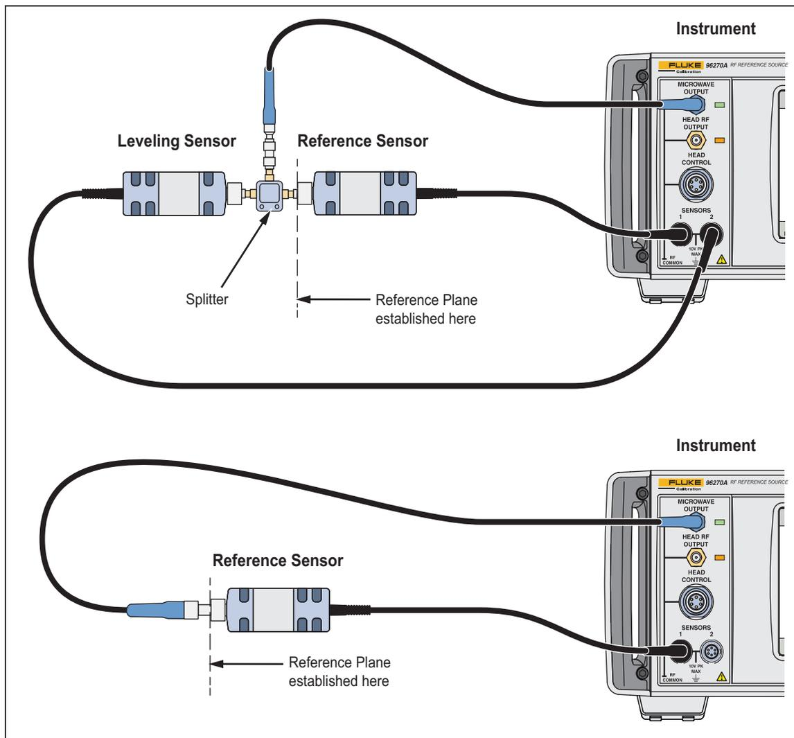
Figure 3-48. Self-Characterization Connections
