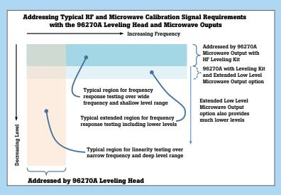
In general, the signals required in RF and microwave calibration can be split into two ranges: at a relatively narrow range of lower frequencies over a wide amplitude range; and at relatively high amplitudes from low to very high frequencies.
