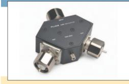
The high current adapter is used when calibrating the A4OB shunts at current levels of more than 2 A. It connects together the current source and two shunts for calibration measurements. This adapter uses LC connectors. In this configuration, a certified or reference shunt is connected in series with a shunt that is being calibrated, which in turn are in series with a current source.
