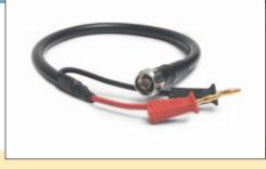
This lead permits connecting the A4OB shunt's N-type connectors to instrumentation that uses dual banana plug connection terminals. Using two leads permits connecting the shunt's voltage output to a voltage measuring instrument and also connecting the shunt's current input to a UUT current source rated 20 A or less.
