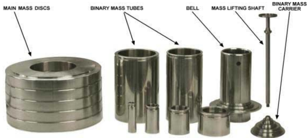
SHOWN IS THE MS-AMH-38 MASS SET FOR THE AMH-38 MASS HANDLER. SMALLER MASS SETS MAY INCLUDE LESS MAIN MASS DISCS. MASS SETS FOR THE AMH-100 MASS SET ARE IDENTICAL TO AMH-38 BUT THE MAIN MASSES ARE LARGER 10 KG DISCS AND A 7TH BINARY MASS TUBE OF 6.4 KG IS INCLUDED.
