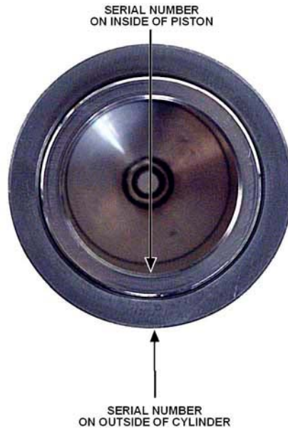
Figure 49. Alignment of the FPG8601 piston in the cylinder
