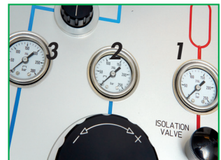
The three pressure gauges indicate: 1. pressure in bottle 2. pressure set by pressure regulator 3. pressure at test port
