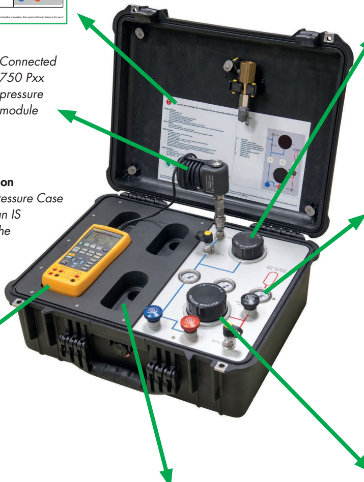
The Minerva MNR 90 precision volume adjuster allows very fine pressure control up to within 100 Pa
