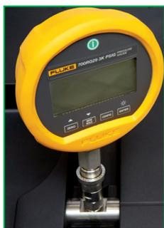
A high pressure swivel connection with quick connector allows the Fluke gauge to be connected and positioned at whichever angle is most convenient for the operator.
