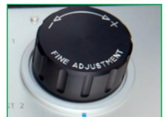
The Minerva MNR 90 precision volume adjuster allows very fine pressure control to within 100 Pa
