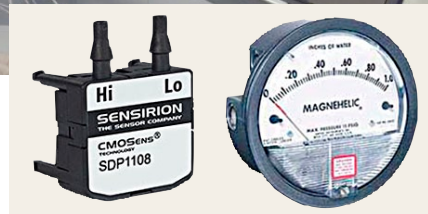
Figure 1. Examples of typical instruments that are used to monitor DP in a clean room environment (Fluke Calibration does not indorse these products).
