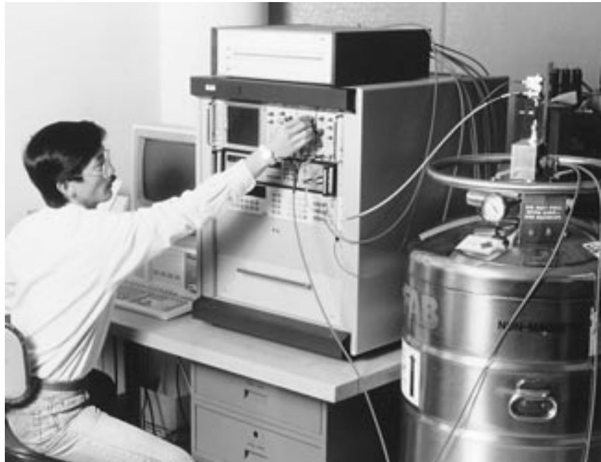
The Fluke DVMP Care Plan offers traceability to its own 10 V Josephson Array, an intrinsic standard of voltage, and to national standards.
