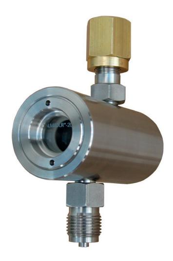
The MNR 140 oil/gas separator is designed to be used with an hydraulic deadweight tester or hydraulic calibrator for testing and calibration of pneumatic instruments up to 300 bar. The MNR 140 has a monitoring glass showing the separation of the fluid and gas. Since there is no diaphragm between the oil and gas inside the unit does not affect the measurement uncertainty of the calibration.
