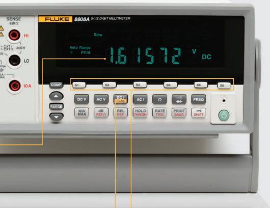
i-Lkg function adds two additional hi-impedance ranges for sensitive low current measurements Setup keys make performing your most common measurements as simple as pressing a button. Increase quality and test times by improving test repeatability by simply saving known measurement setups to front panel accessible setup keys. All the operator has to do is select the right setup key.
