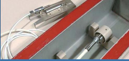
Control of temperature and shrinkage in High Temperature drying processes of bricks, tiles and ceramics. (up to 250°C)
