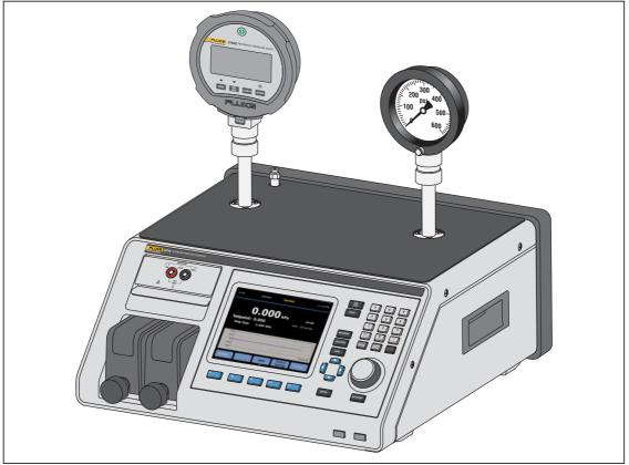
Figure 4. Two Gauge Connection
