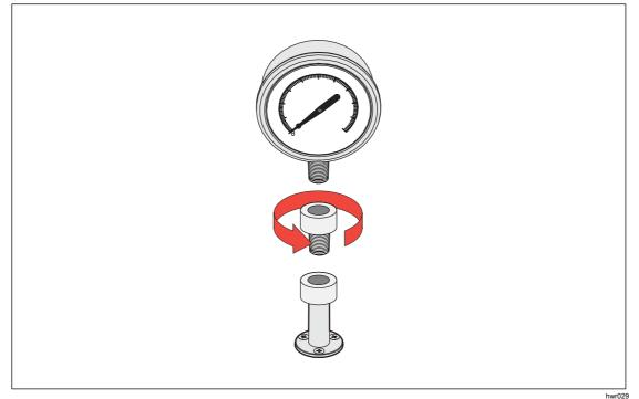
Figure 6. Screw on Gauge Adapter
