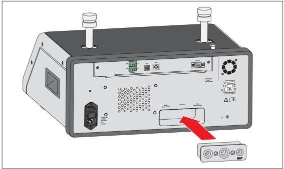
Figure 29. Manifold Installation
