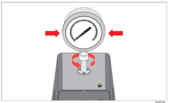
4. Hold the instrument steady, while turning the gauge adapter COUNTER-CLOCKWISE until it pulls down onto the O-ring, see Figure 21.
