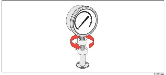
Figure 7. Connect Assembly to Test Port
