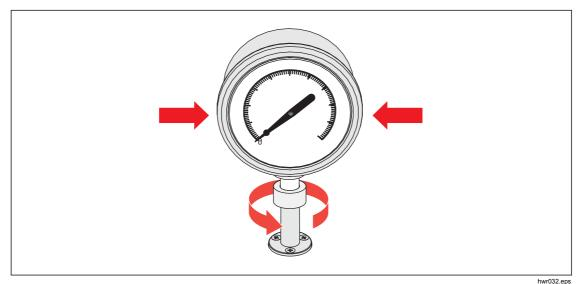
4. Hold the instrument steady, while turning the gauge adapter COUNTER-CLOCKWISE until it pulls down onto the O-ring, see Figure 9.
