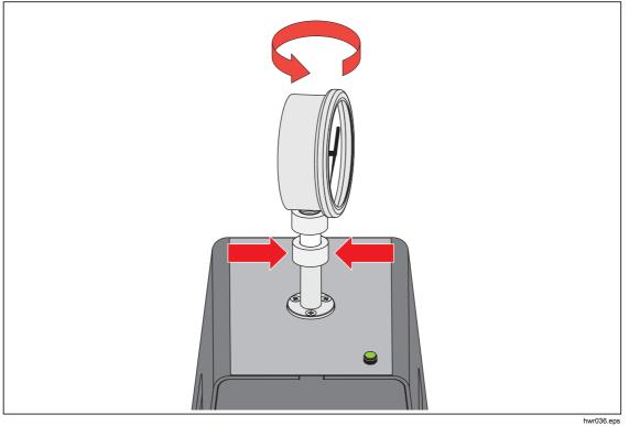
3. To adjust the position to face forward, hold the gauge adapter and turn the instrument COUNTER-CLOCKWISE, so that it faces forward, see Figure 20.
