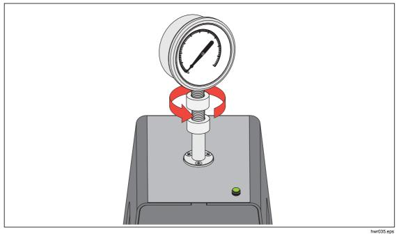
Figure 19. Connect Assembly to Test Port
