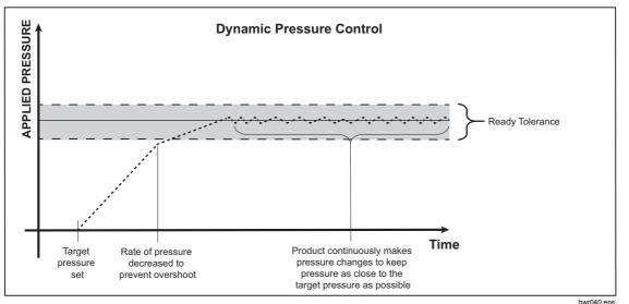
Figure 11. Dynamic Pressure Control Mode Example
