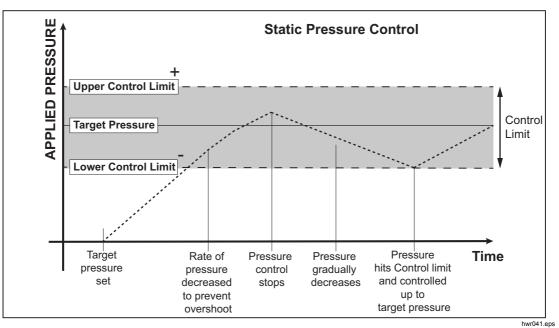
Figure 12. Static Pressure Control Mode Example
