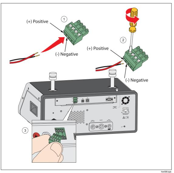
Figure 27. Driver Connections
