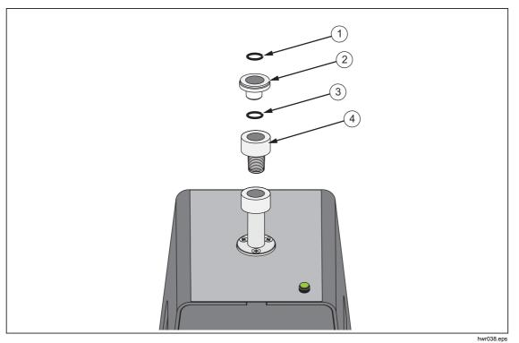
Figure 22. Test Port Insert
