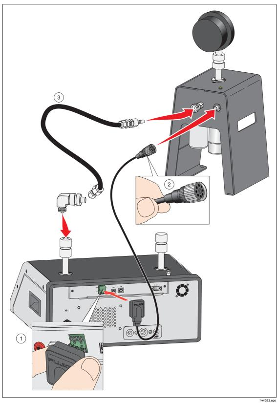
Figure 17. CPS Driver and Manifold Connections
