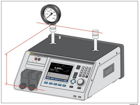
Figure 13. Head-Height Correction Measurement
