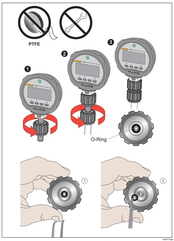
Figure 5. Replacing M20 O-ring
