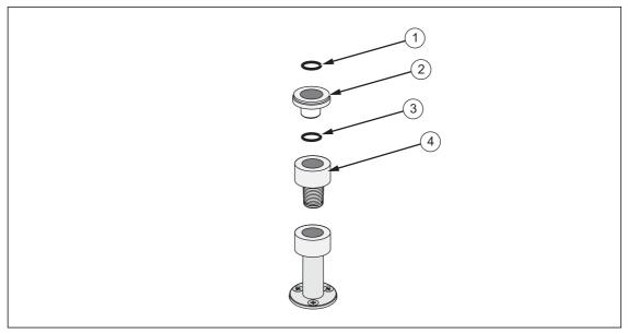
Figure 10. Test Port Insert
