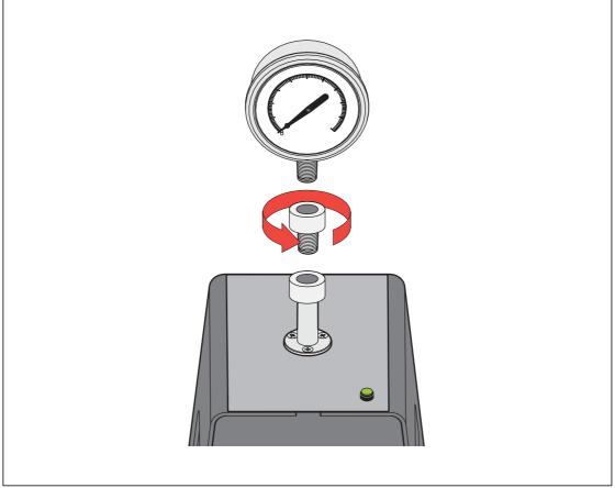
Figure 18. Screw on Gauge Adapter
