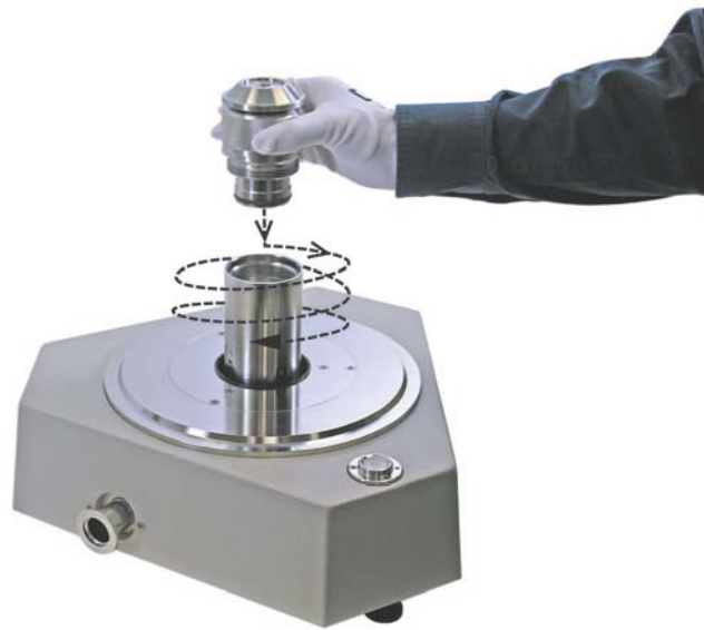
Figure 4. Piston-Cylinder Module Installation
