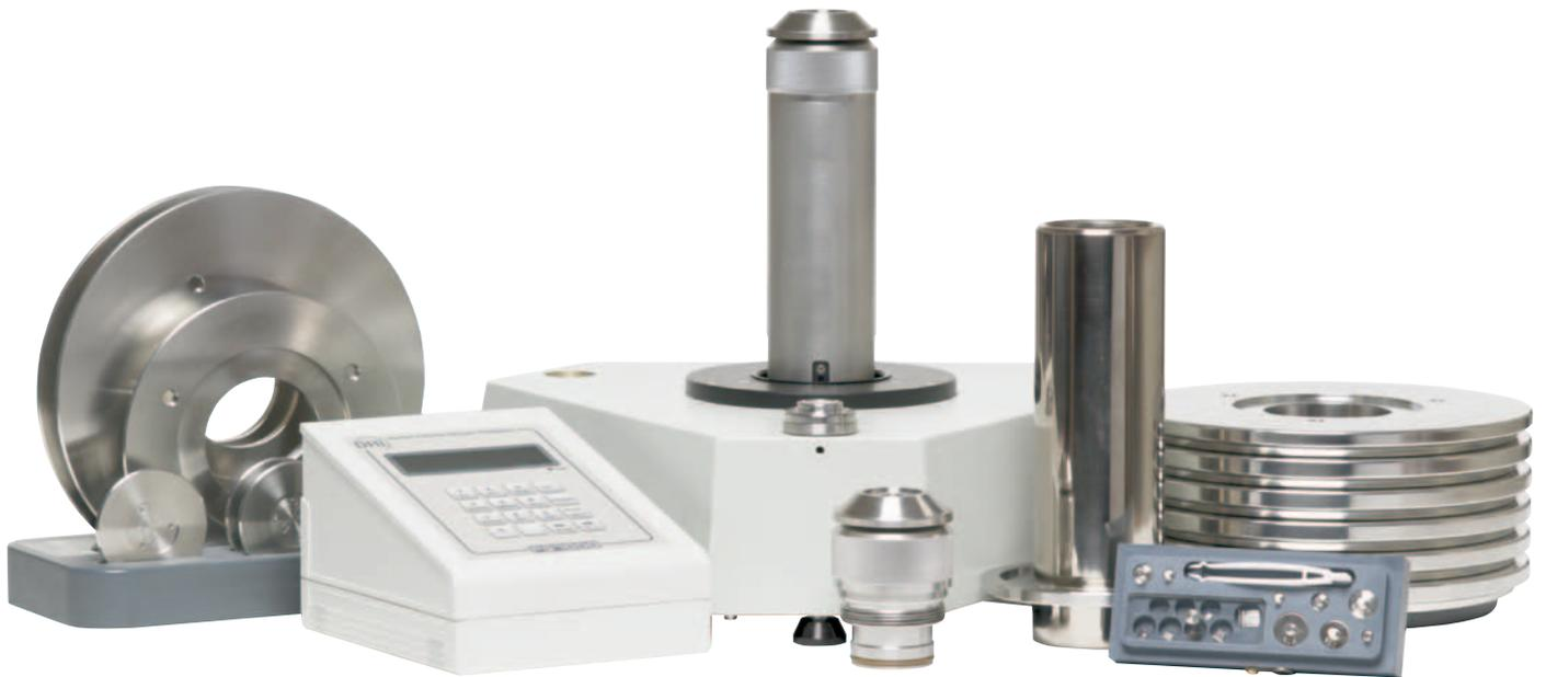
The piston gauge's fundamental operating principle and excellent long term stability have made it an indispensable tool in high accuracy pressure metrology. As accuracy levels increase, quality assurance requirements intensify and automation spreads through the workplace, the piston gauge must evolve to continue to fill its essential role in the measurement system. PG7000, the first truly new, high end piston gauge introduced since the late 1970s, responds to this challenge.
