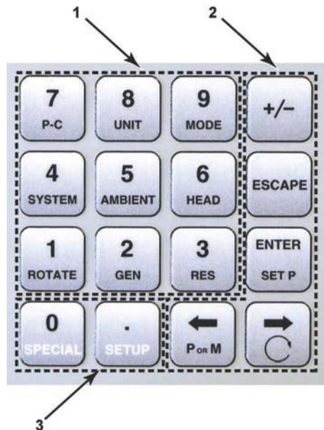
1. The **Function/Data keys** allow very commonly used functions to be accessed directly from the main run screen by a single keystroke. The name of the function is on the bottom half of the key (see Section 4.3). These keys enter numerical values when editing.
