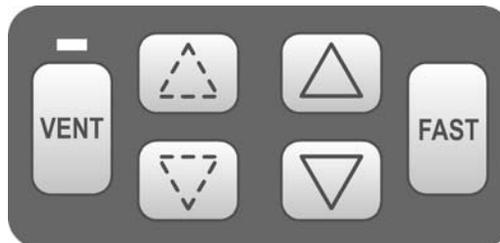
**Figure 20.** Pressure controller direct pressure control keys
