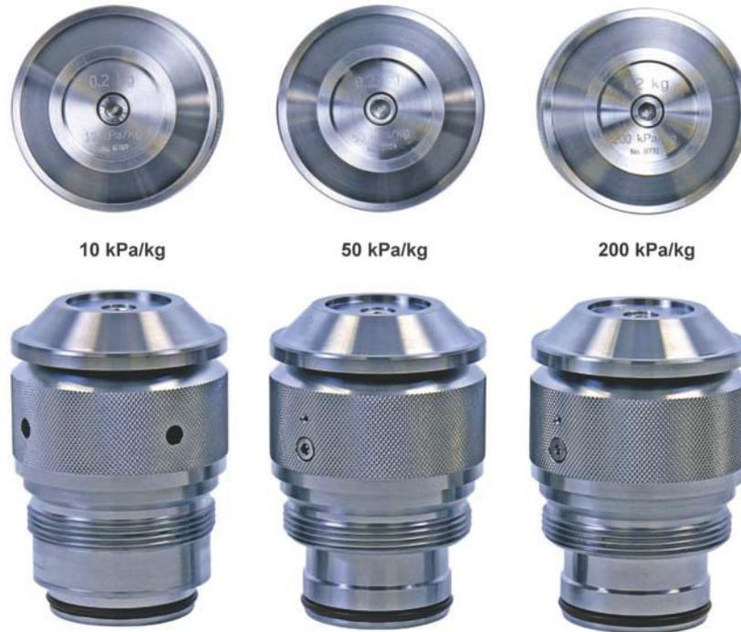
**Figure 8.** Piston-cylinder modules, PC-7100/7600-10-L, -50, -200
