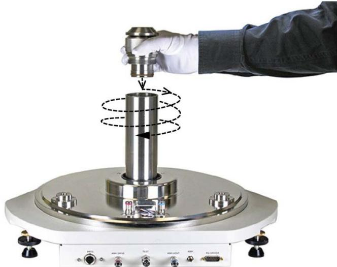
Figure 11. Piston-Cylinder Module Installation
