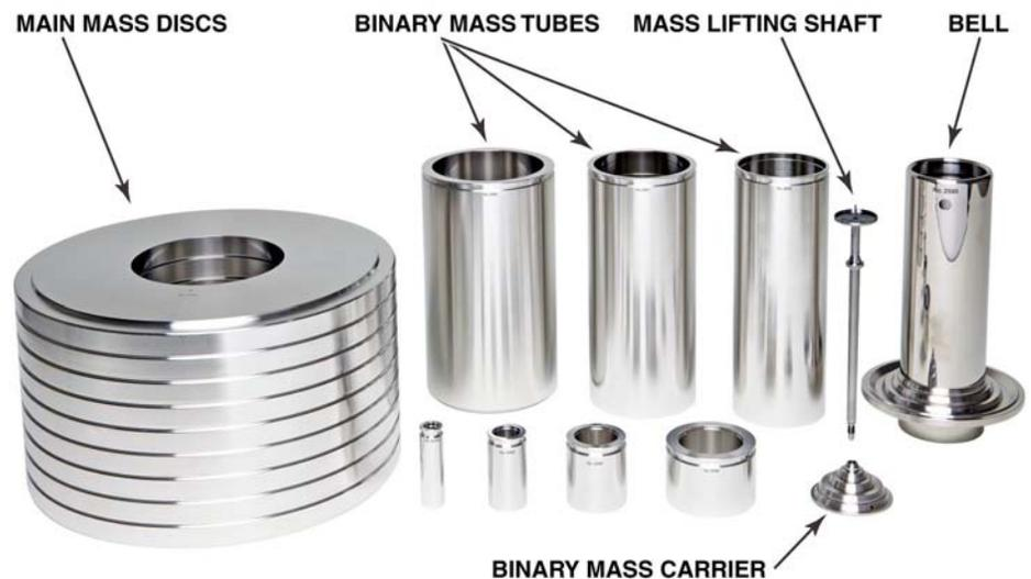
Shown is the MS-AMH-100 mass set for the AMH-100-VAC mass handler. Smaller mass sets may be used with AMH-100-VAC which include fewer main mass discs.
