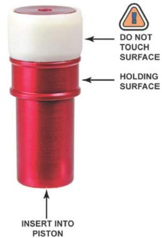
**Figure 25.** 10 kPa/kg piston insertion tool
