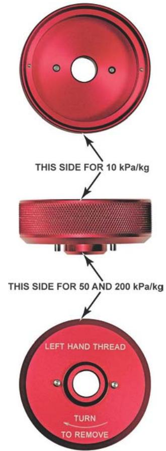
**Figure 24.** Gas piston-cylinder module sleeve nut tool
