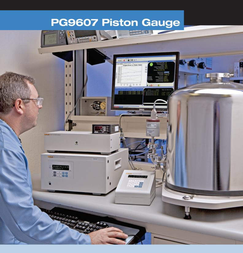
Automated primary pressure reference for absolute and gauge pressures to 500 kPa
