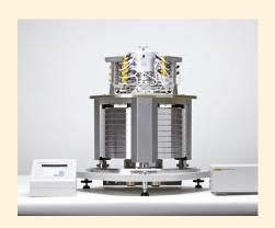
The DH Instruments PG9607 is the next generation of absolute pressure piston gauge from Fluke Calibration. It supports the use of a 100 kg mass set to define gauge and absolute pressures from 11 to 500 kPa with a single piston-cylinder.
