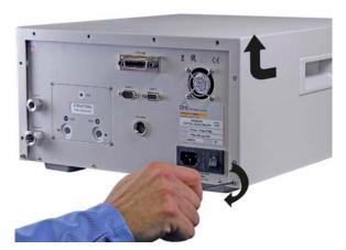
Figure 1: Removing the PPC4 Chassis Cover
