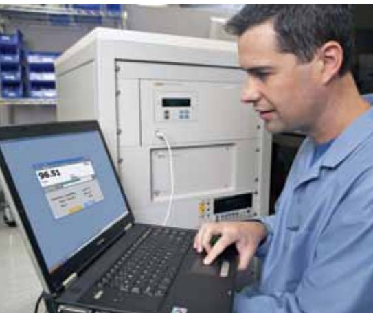
PPC4 standard front panel USB connection provides easy access and use of "cockpit" software for full PC based plug-and-play functionality
