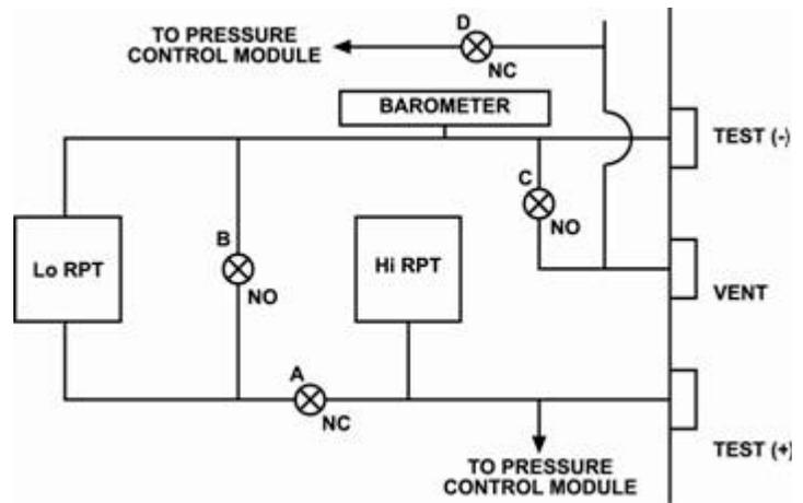
**Figure 18.** PPC4E Reference Pressure Transducer Module Schematics
