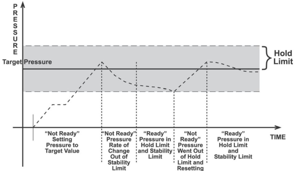
Figure 6. Ready/Not Ready in Static Control Mode
