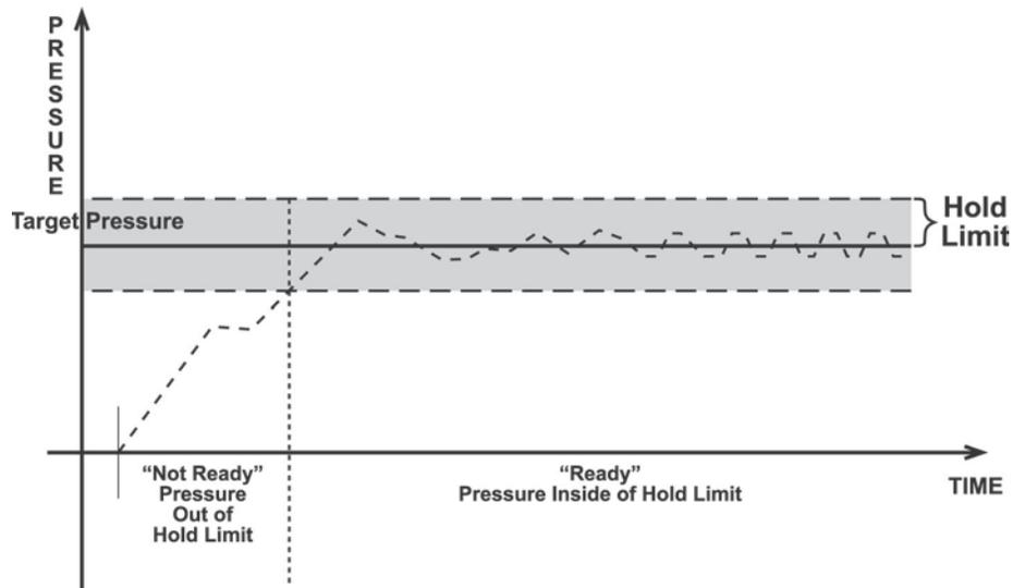
Figure 5. Ready/Not Ready in Dynamic Pressure Control Mode
