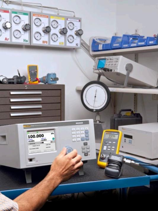
Uncertainty of the measured or delivered pressure is calculated and displayed continuously by PPC4E. The calculation uses uncertainty components based on PPC4E specifications and the component values can be tailored by the user.
