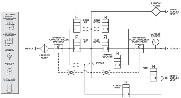
Figure 17. Pressure Control Module Schematic
