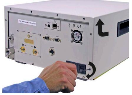
Figure 15. Removing Back Cover
