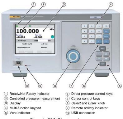
Figure 1. PPC4E front panel
