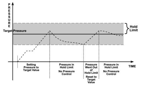
Figure 4. Static Pressure Control Operation
