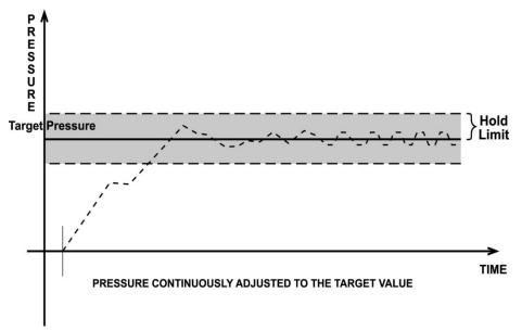
Figure 3. Dynamic Pressure Control Operation
