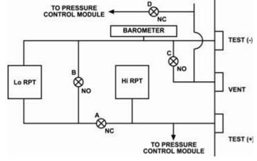
Valve D is shown for reference. It is in the pressure control module. Valve C is the TEST (-) vent valve. In normal operation with PPC4EX 100K, this valve is closed during fine pressure control (see Section 3.5.7.5).
