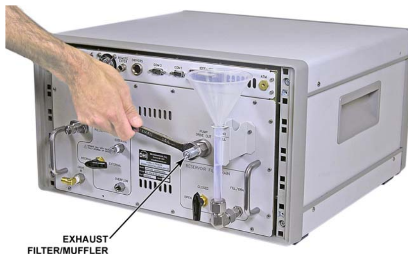
Figure 5. Installing the exhaust filter/muffler
