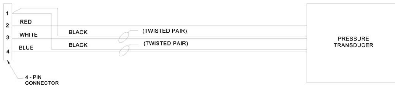
Figure 2: RPM3 Components and Transducer Wiring Diagram
