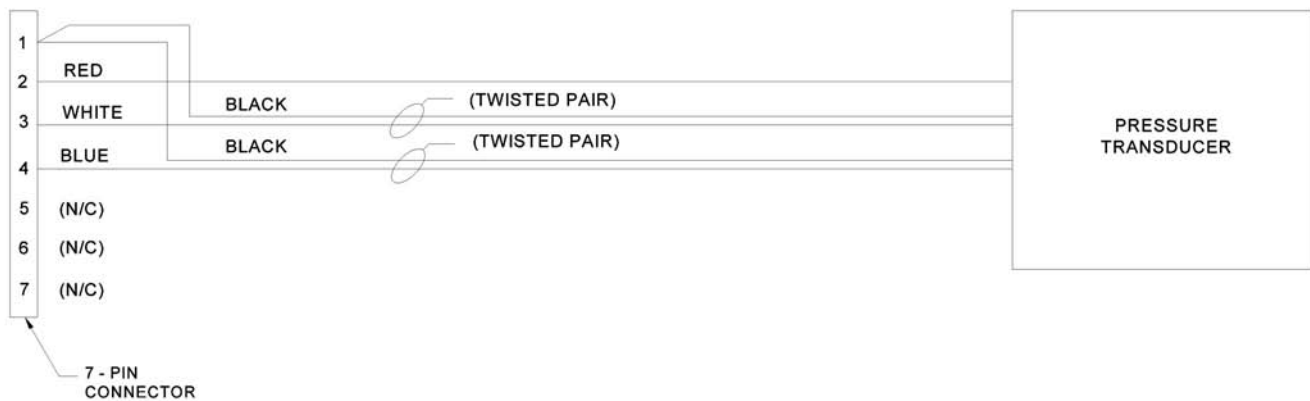
Figure 5: RPM4 and PPC3 Components and Transducer Wiring Diagram
