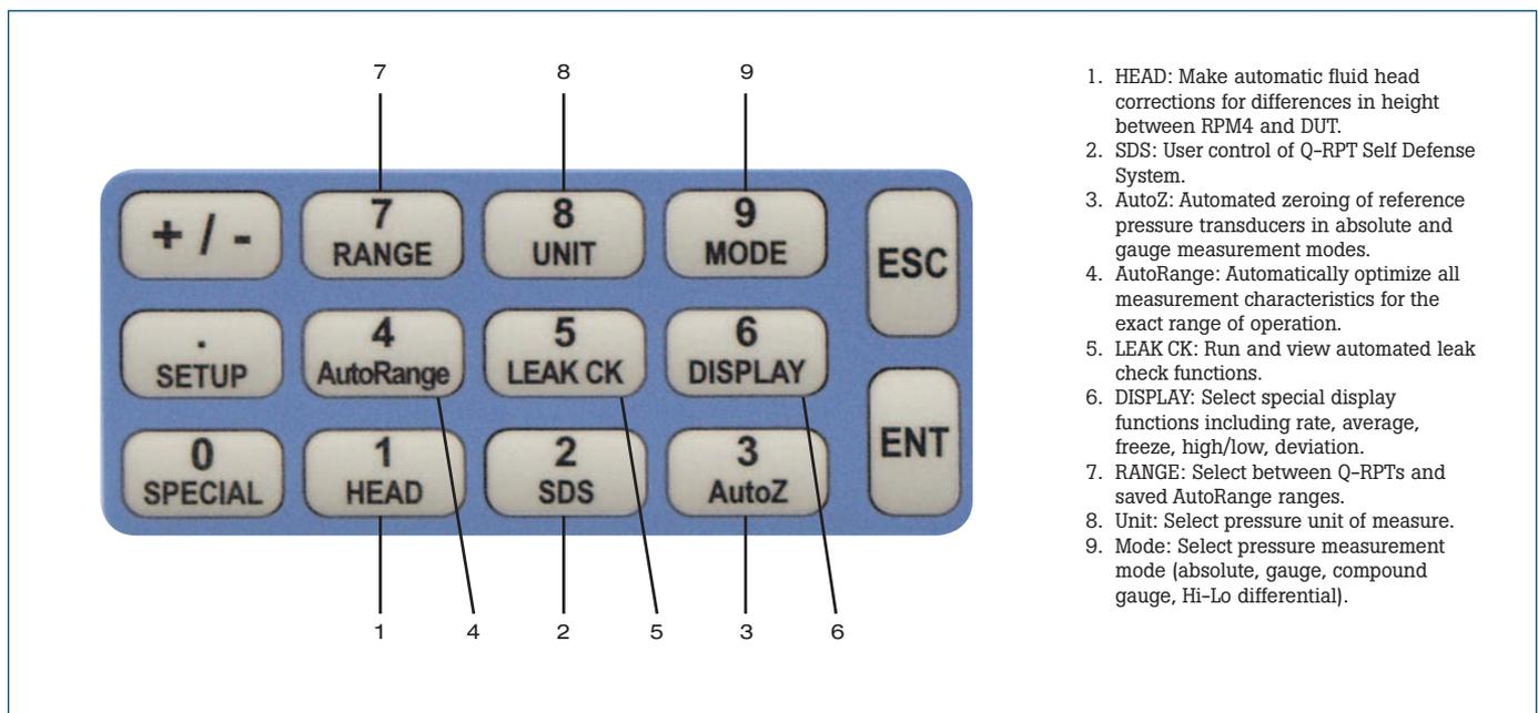
1. HEAD: Make automatic fluid head corrections for differences in height between RPM4 and DUT.
