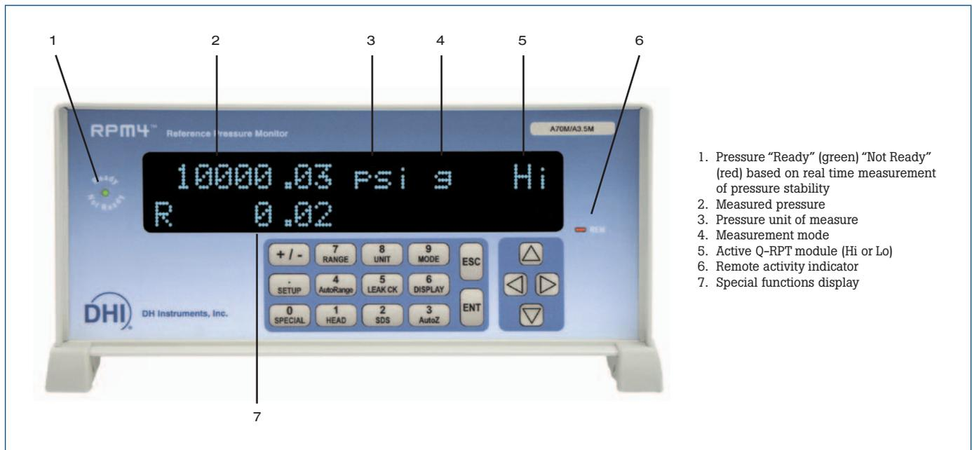
1. Pressure "Ready" (green) "Not Ready" (red) based on real time measurement of pressure stability
