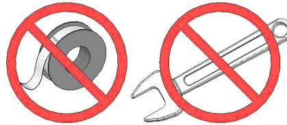
Figure 13. Do Not Over Tighten
