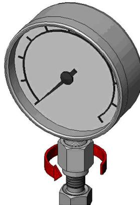
**Figure 8. Screw on Gauge Adapter**
