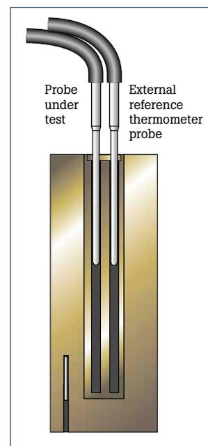
Maximum accuracy for short probes can be obtained by comparing to a similar probe at the same well depth.
