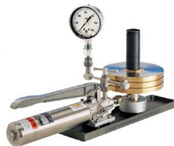
Figure 2. A conventional deadweight tester generates, controls, and measures hydraulic pressure.
