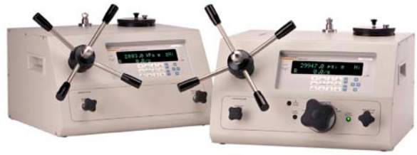
Figure 4. The E-DWT-H Electronic Deadweight Tester from Fluke Corporation, DH Instruments Division, is a single piece solution for calibrating high pressure hydraulic gauges. The H indicates hydraulic platform.
