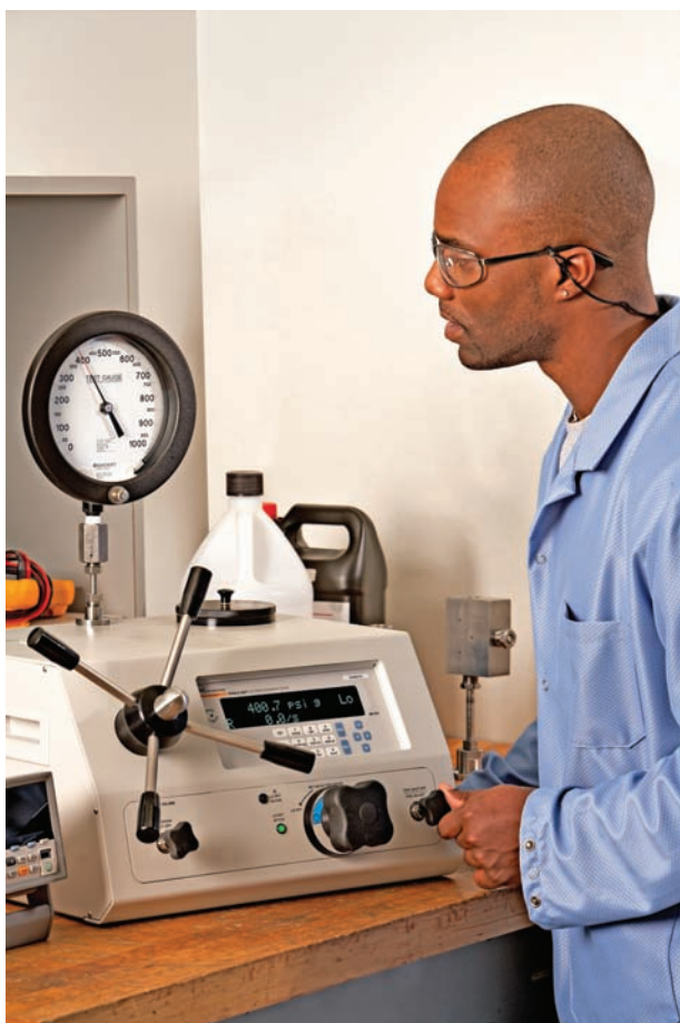
Figure 5. E-DWT-H's fine adjustment valve enables the operator to set pressure to the exact nominal value on the gauge under test.
