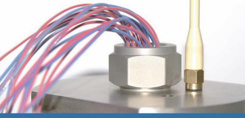
Measurement of temperature inside your thermal cycles under pressurized atmosphere with a real time thermocouple logger and/or transmitter.
