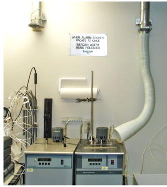
Figure 1 Ventilation system for removing oil vapors.
