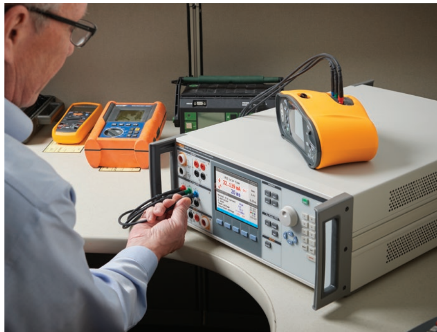
Each 5322A comes with an external R-Multiplier to source resistances of 10 TΩ for testing insulation testers.
