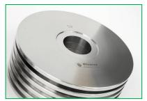
The mass set composition is such, that any desired mass value within the mass set range can be loaded within 0.01 g.
