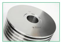
The mass set composition is such, that any desired mass value within the mass set range can be loaded within 0.01 g.
