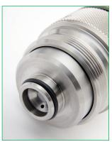
The piston-cylinder defines effective area and is the piston gauge's principal metrological element. The piston-cylinder's intrinsic characteristics and how it is mounted and exploited are the keys to piston gauge performance.
