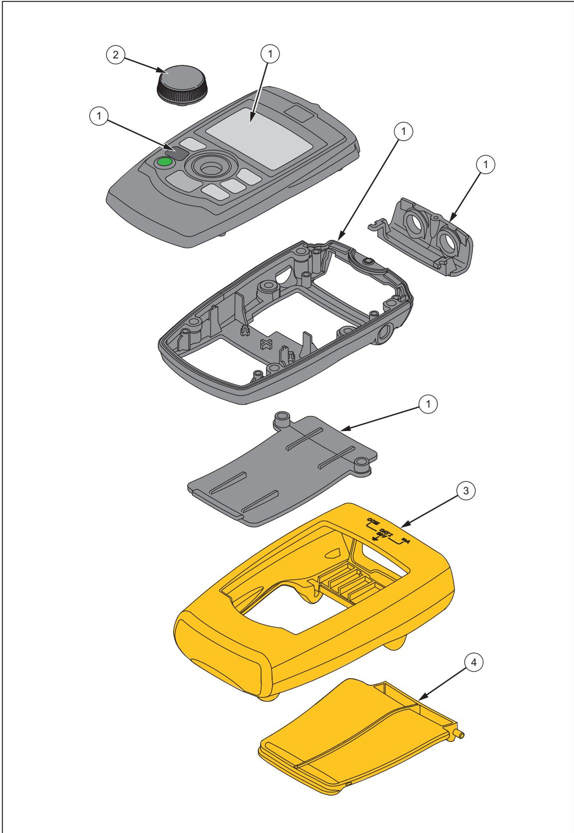
Figure 6. User-Replaceable Parts
