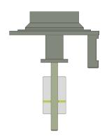
The piston cylinder systems for pneumatic operation with liquid lubrication have a groove set into the inner bore to which liquid is supplied through two radial holes.
